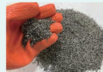
Recycled polyvinyl chloride (Eco-Flake) manufactured from waste tile carpet
