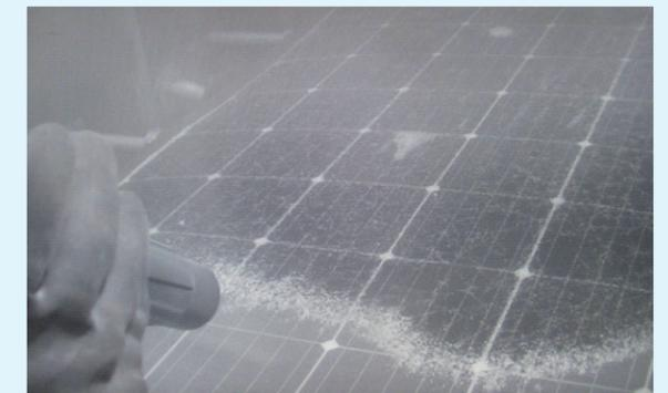
Crushing and separating an used solar panel glass
