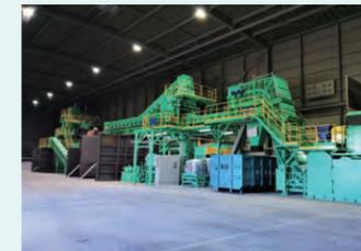
Sorting and crushing line for combustible materials, which includes optical sorters at the Kawasaki Recycling Center.
