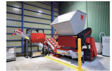
Shredding and magnetic sorting line (REVER CORPORATION's ELV Kawajima Plant)
