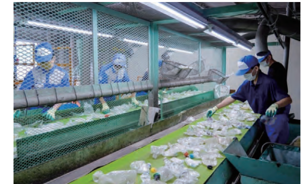
The plastic bottle sorting process
