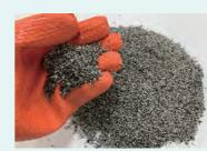
Recycled polyvinyl chloride (Eco-Flake) manufactured from waste tile carpet
